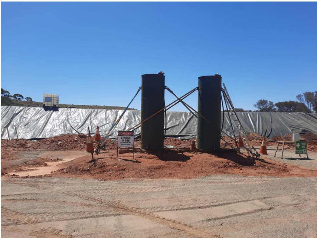
Figure 7: Carbon Tanks in situ at East Menzies extracting and holding onto precious metals, December 2024
