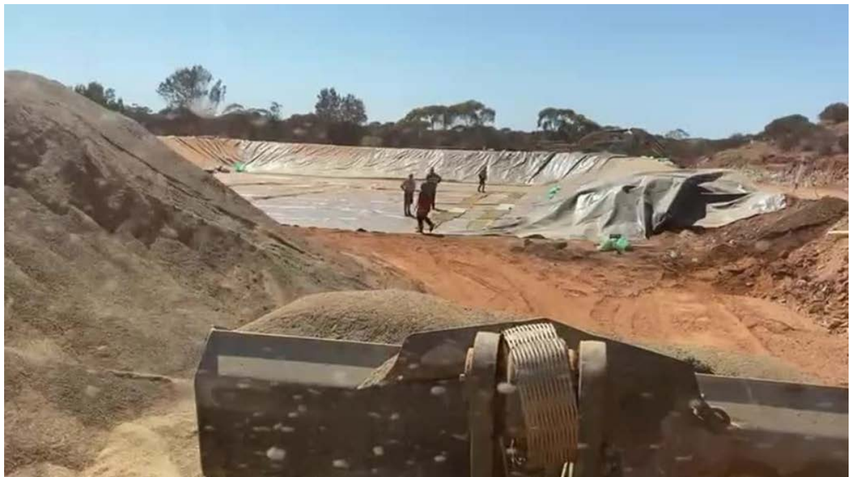
Figure 5: Crushed material about to be loaded into the vat leach facility at East Menzies Gold Project, November 2024
