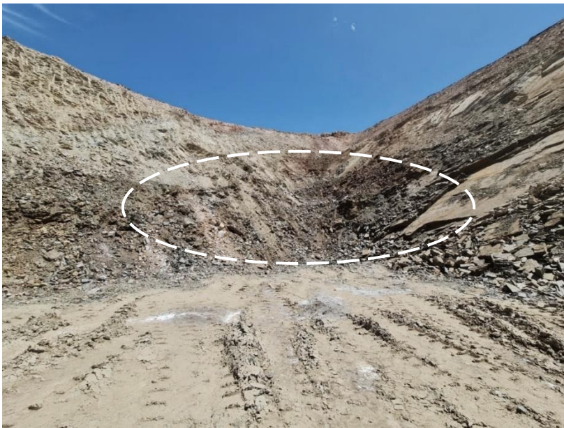
A picture of the Jeffreys Find ore body showing gold mineralisation evidenced by darker zones
